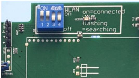
**Switch 1** - The Wi-Fi switch in **ON** position allows communication with the electronic card using a smart phone. The on-board Wi-Fi access point is available for accepting connections.
