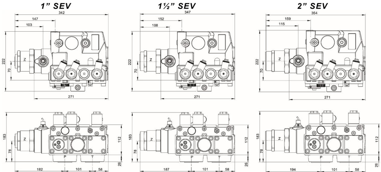
Figure 3: SEV valve dimensions
