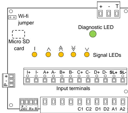
Pro-Hydro card includes 5 yellow signal LEDs and a diagnostic LED. The yellow LEDs light up when corresponding input signals are received. The Diagnostic LED changes its color and blinking pattern according to the failure status. This is given in below table.
