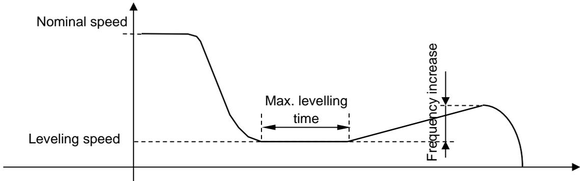
Figure 38: Leveling recovery function
