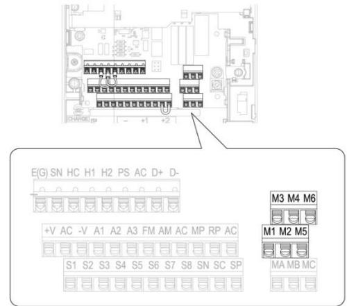
Note that the allowed voltage and current for the outputs are restricted to 30 VDC / 250 VAC / 1 A. See the inverter technical manual for more details.
