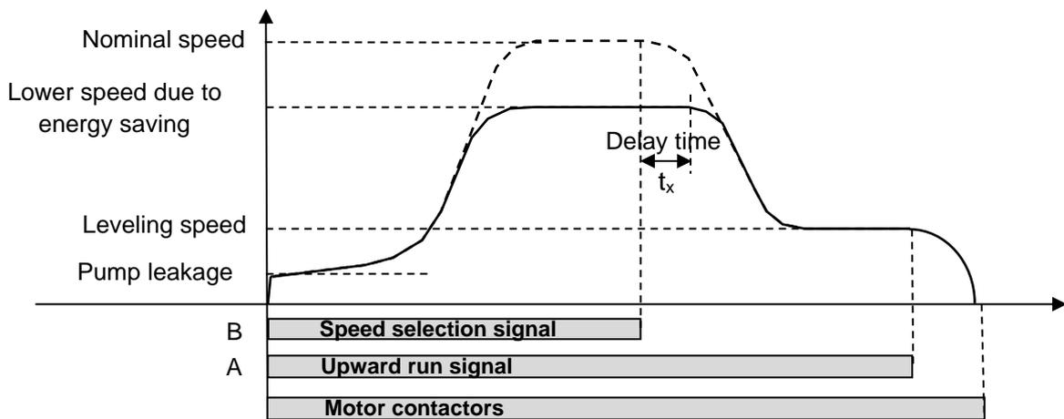
Figure 37: Deceleration compensation to have constant leveling time
