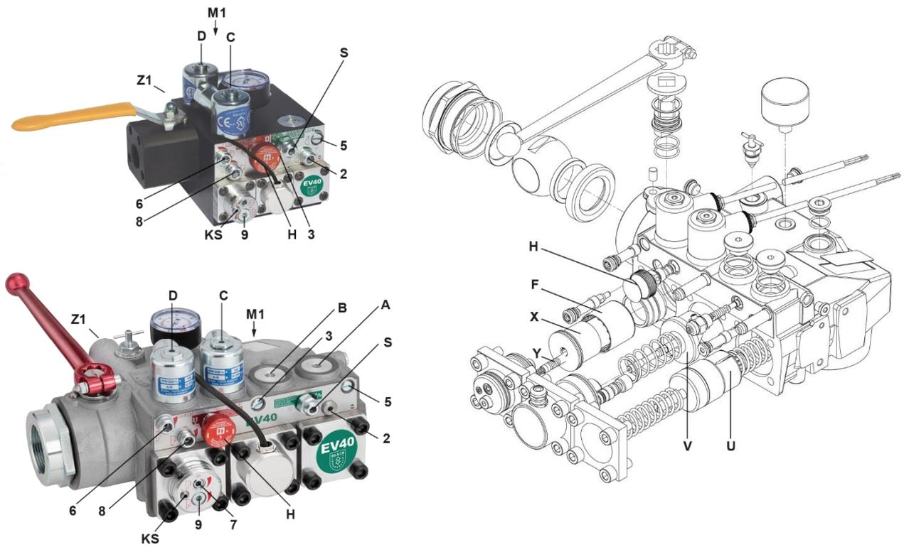
**Figure 5: EV40 adjustments and explosion drawing**
