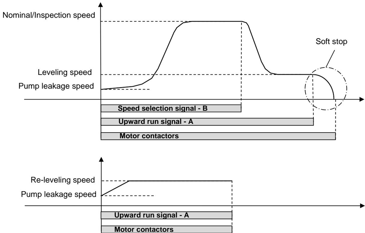
Figure 36: Signaling the drive for different travels
