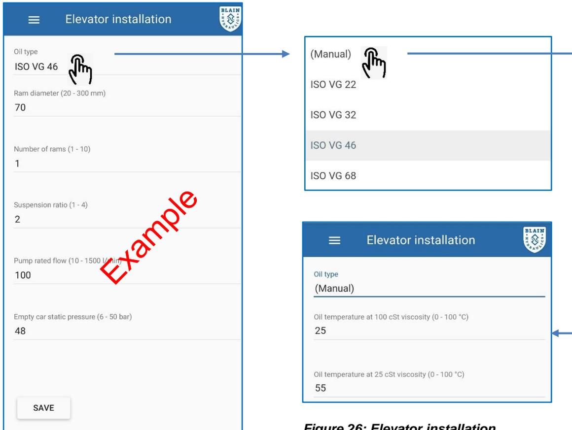
**Figure 26: Elevator installation**
