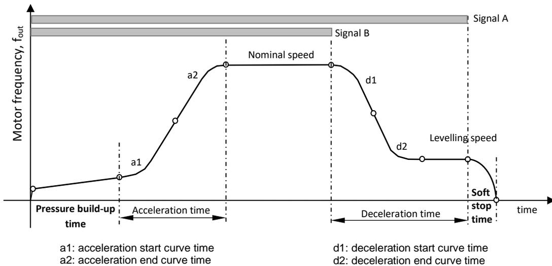
**Figure 34: Target parameters**
